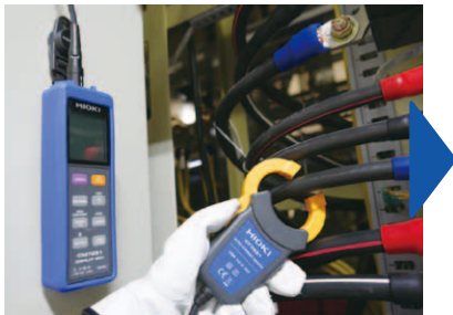
Connect the sensor to the Display Unit CM7291 and clamp in around the cable to be measured.
